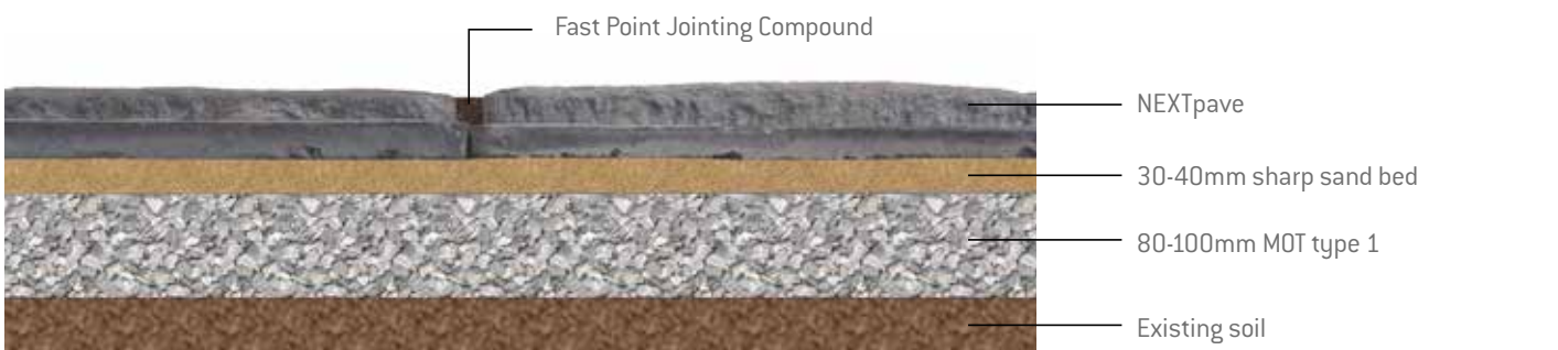
4. Install the engineered NEXTpave using the laying pattern
